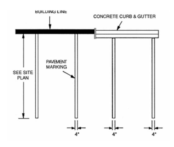
Layout and paint all parking bays and roadway markings using heavy-duty maximumlight reflective traffic paint that meets or exceeds Federal specifications.
